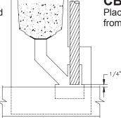
**CB-6** Place bus bar into mold Tap cable is gapped 1/4" from upper edge of bus bar.
