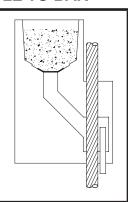
CB-2 Place bus bar into mold Tap cable is gapped
